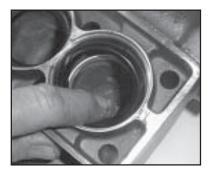
10. Place support ring (41) and v-sleeves (40) into valve casing.
